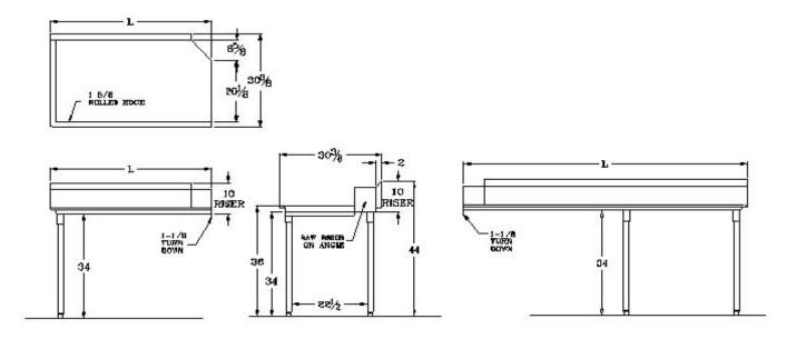
All units ship unassembled for reduced shipping cost. Units 7 ft. and larger are furnished with four legs.
